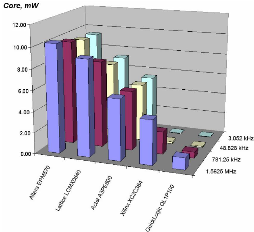
1. Power measurements are for the core VCC supply only, and do not include any auxiliary or I/O power supplies.
