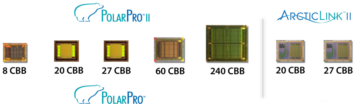
Figure 3: The QuickLogic PolarPro, PolarPro II, ArcticLink and ArcticLink II Solution Platforms offer a wide range of fabric capacities.
